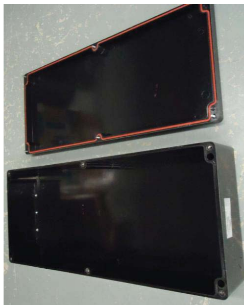
Picture 6: Polymeric enclosure, Model No. QX-P, Internal view
